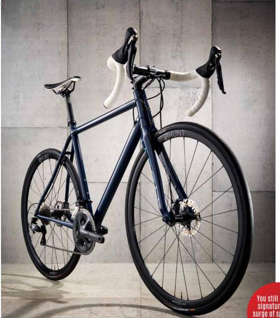
Below Shimano disc brakes with 140mm rotors keep the Mason under control **Bottom** MultiPort inserts make for neat internal cable routing
