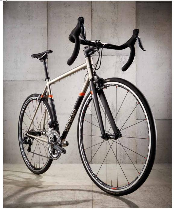
Below BB86 Press-Fit bottom bracket provides a stiff, efficient pedalling platform Bottom Gearing is a mix of Shimano Ultegra Di2 and FSA kit
